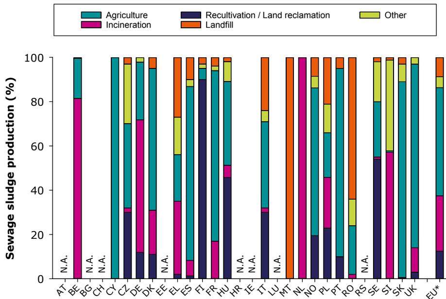
Figure 25: Destination of the sewage sludge production
